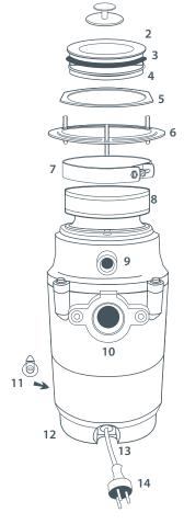
Fig 1. Three Bolt Mount System
